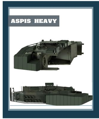
The ASPIS (Advanced Shielding Platform Integrated System) is appropriately designed to equip future combat vehicles and existing MBT that need to be upgraded. The turret model demonstrates the layout of a modern multi-layer active and passive ballistic (hybrid) armor, protecting against current and future battlefield threats as long rod penetrators and top-attack threats.
